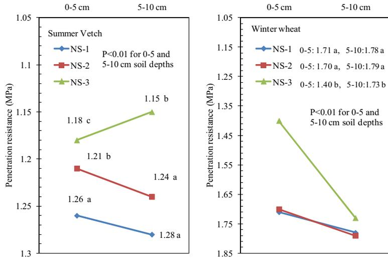
**Figure 3-Effects of no-till seeders on the penetration resistance**
