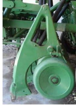
Hoe type furrow opener for the Amazone/NT 250 No-till seeder. Direction of forward travel is right to left
